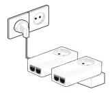
A simple way to check if both adapters are connected is to plug both adapters side by side into a power strip. Now connect the power strip to the mains. If both adapters form a network, the PLC-LED (depending on the product in use  $\hat{\mathbf{L}}$  or o) will light up permanently white.
