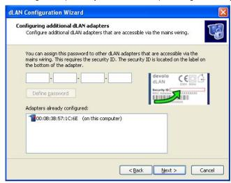
Once you have entered the security IDs of your dLAN adapters, your dLAN network is complete. All computers and other network devices connected to the adapters by cable should now be able to communicate with one another in the network
