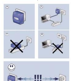
Also position the adapter away from your computer, as it may interfere with the adapter's operation.  Plug the devices into different outlets and avoid using the same extension strip.
