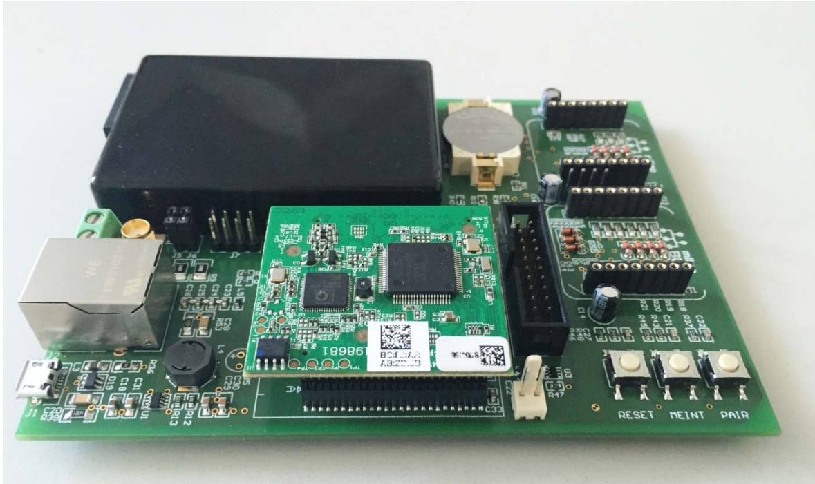
Fig 2: Picture of the devolo dLAN® Green PHY eval board II (side view)
